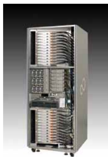
Fig. 2. K-Computer rack. Computing nodes are mainly cooled by water, but memory, system board, power supply units and other components still need air cooling.
