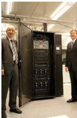
Fig.1. System IBM Aquasar with water cooling. As it requires heat exchange modules, pumps, and space for water conduits, the power density is lower than for the air cooled IBM blade system.
