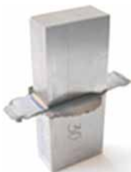
Fig. 2. A sample of a linear friction welding joint
